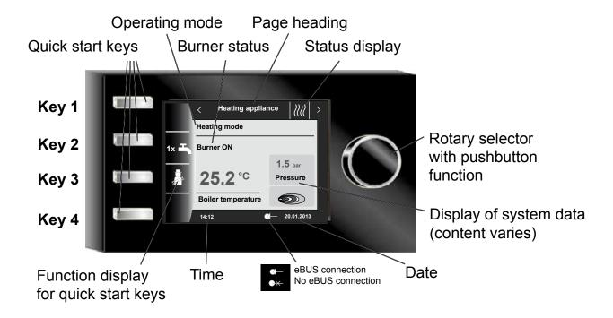
After switching on the heating appliance, the software loads, and a progress bar and the Wolf logo appear. The system is then initialised and the system is reloaded. The start page / home page is now displayed.
